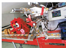
Once baked, I use a wrapping machine to put the wrappers on.
